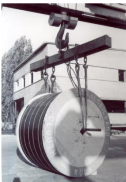
Conveyor belt transport onto lorry
